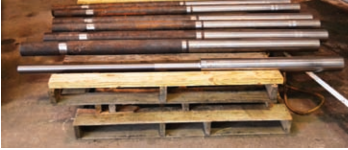
3-1/2" O.D. 4340 steel alloy material for the anti-spin shaft.
