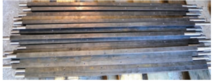
Square shafts with drilled and tapped holes using the Ganesh VFM 6237 Machining Center equipped with a Mitsubishi control and 30 HP spindle motor.
