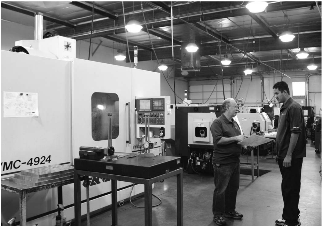
Dan Dasher, left, shop foreman, and machine operator Bartolo Assero discuss a job to be run on Transco's Ganesh VMC-4924 vertical machining center. The machine is one of 6 Ganesh machines operated by Transco. The other 5 are Cyclone, Swiss-style turning centers. The heavy-duty VMC-4924 features a triple linear way system and rapids of 1,181 inches/minute.
