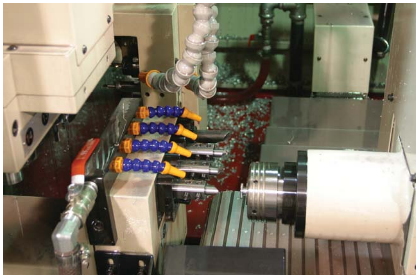
Close up inside the new Ganesh Cyclone CS32 7-axis, live-tool Swiss-style turning center. Subspindle is on the right-hand side.
