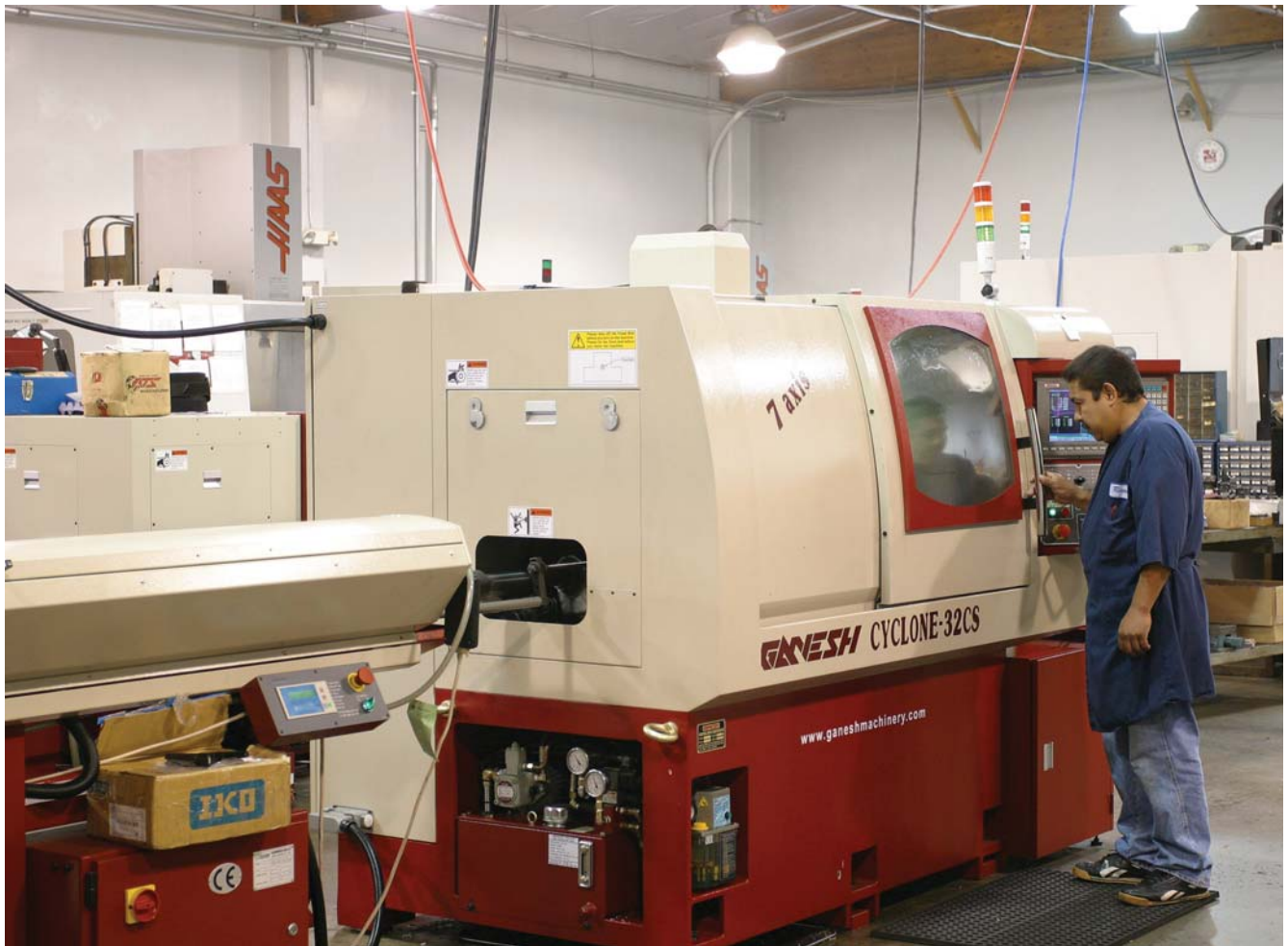
Ricardo Espinoza, CNC machine operator, sets up Transco's new Cyclone-32CS 7-axis CNC Swiss-style turning center. The machine has simultaneous sub-spindle with full C-axis, 32 tools, 7 live stations on the main spindle, 6 stationary turning tools, 5 drill, tap and bore tools for end working, 9 back-working tools on the subspindle (4 Live), 1.25" diameter bar capacity, a Fanuc-compatible PC-based graphical control, sliding head stock without a guide bushing, hydraulic collet chuck, 10-hp main spindle, 5-hp subspindle, programmable parts catcher with part draw, automatic lubrication system, a coolant system with chip filtration, and a chip conveyor system with chip cart.
