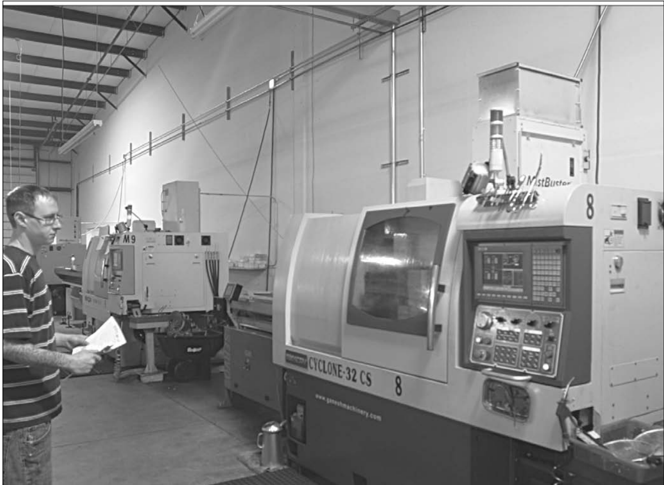
Inspector John Pope approaches a lineup of three of four Ganesh Cyclone-32 CS lathes at Owens Precision.
