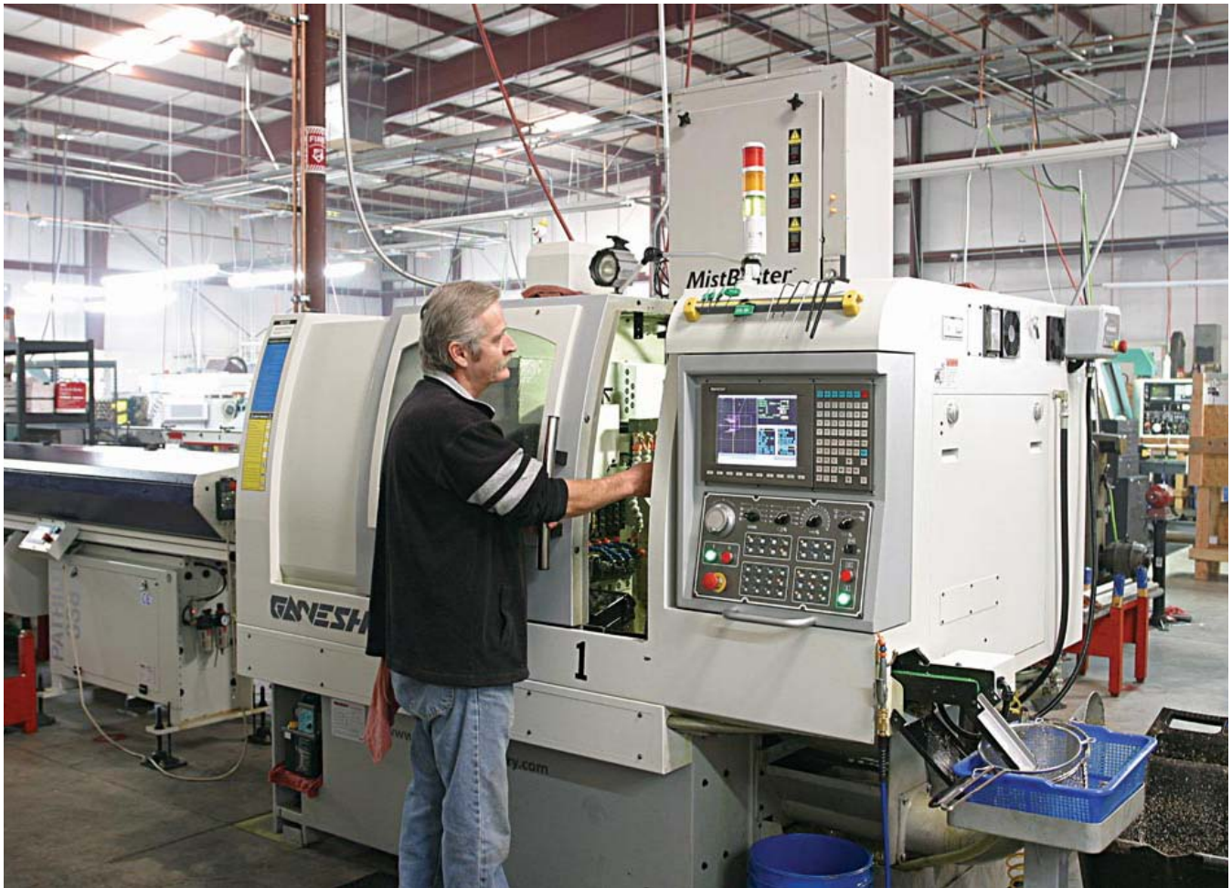
Machinist Allen Seals sets up Owens Precision's newest Ganesh Cyclone-32 CS lathe. The lathe features a total of 27-tool stations. The main spindle uses 18-tools, which are comprised of a bank of 4-live cross tools, a bank of 3-axial live tools, 6-turing tool stations, and 5-ID tool stations, all in a gang configuration. Bar feeder is an Edge Technology Rebel multibar feeder.
