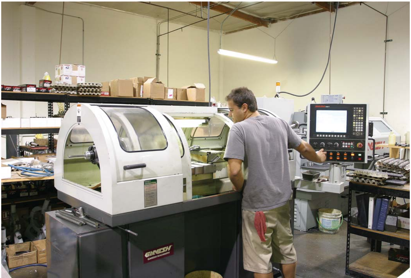
CNC machine operator Jimmy Spoto sets up a Ganesh CNC 610 gang tool lathe, Radflo's latest purchase.
