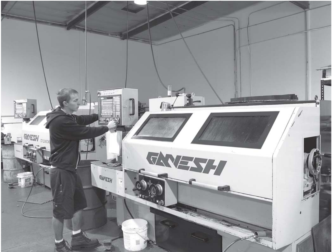
Operator Ryan Evelo prepares to run parts on one of two Ganesh GT-2050 CNC lathes owned by Radflo Suspension Technology. In the background is a GT-2040 machine. Both machines feature Fagor 8040 conversational controls.
