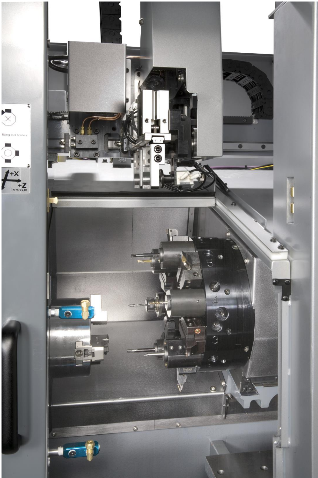
BMT-55 Driven Tool Turret Standard. Optional VDI-30 Driven Tool Turret pictured above.
